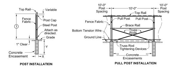
Place fence fabric on roadway side of post. For certain curves, stream crossings, or other locations, the Contractor has the option to place fabric on the side of the post away from the roadway.
