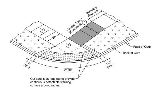
1 Parallel Curb Ramp: If normal sidewalk elevation cannot be achieved with the perpendicular ramp between the street and landing due to limited ramp length, provide a parallel ramp to make up the elevation difference between the landing and the standard sidewalk.
