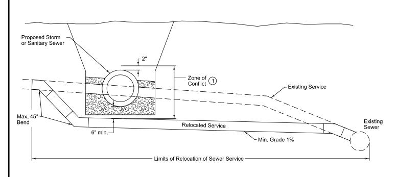
2 Zone of conflict is from 6 inches below the bottom of sewer pipe to 2 inches above the top of pipe.
