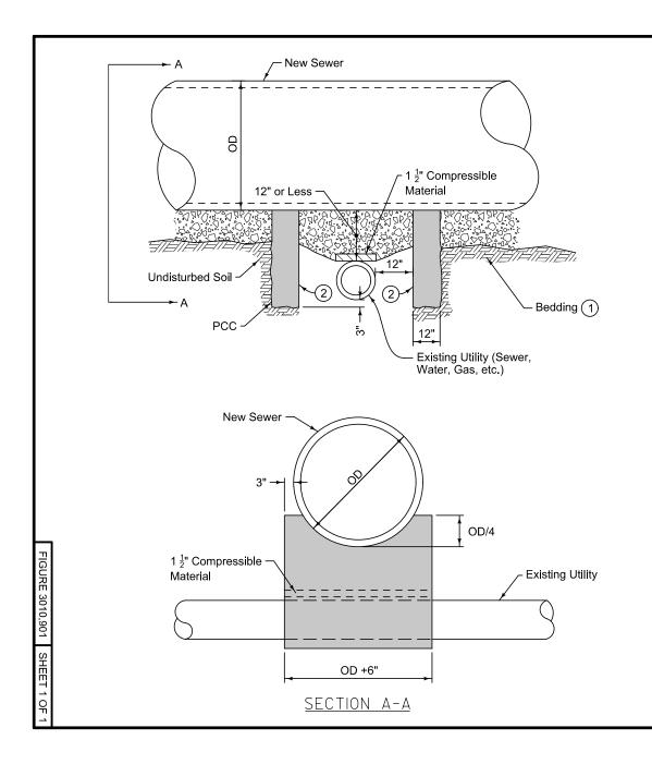
Install pipe support for all new sewers 12 inches in diameter or larger when clearance between bottom of new sewer and top of existing line is 12 inches or less.
