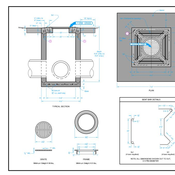
Top of intake may be poured in the field or precast. For precast units, place a 1 inch diameter X 3 inch deep alignment hole 3 inches from each side of the corners of the unit.
