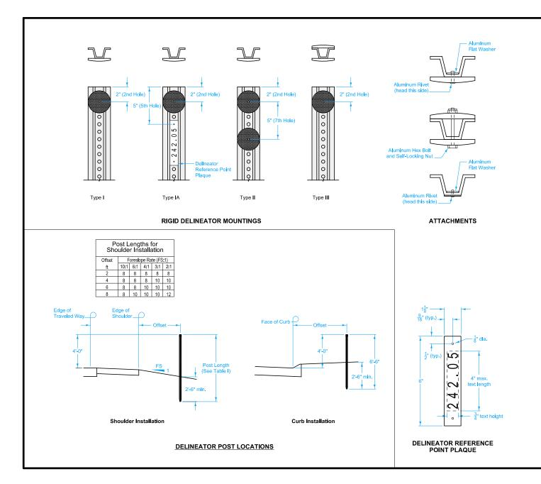
Place delineators at a constant distance from the edge of traveled way and/or the edge of shoulder.
