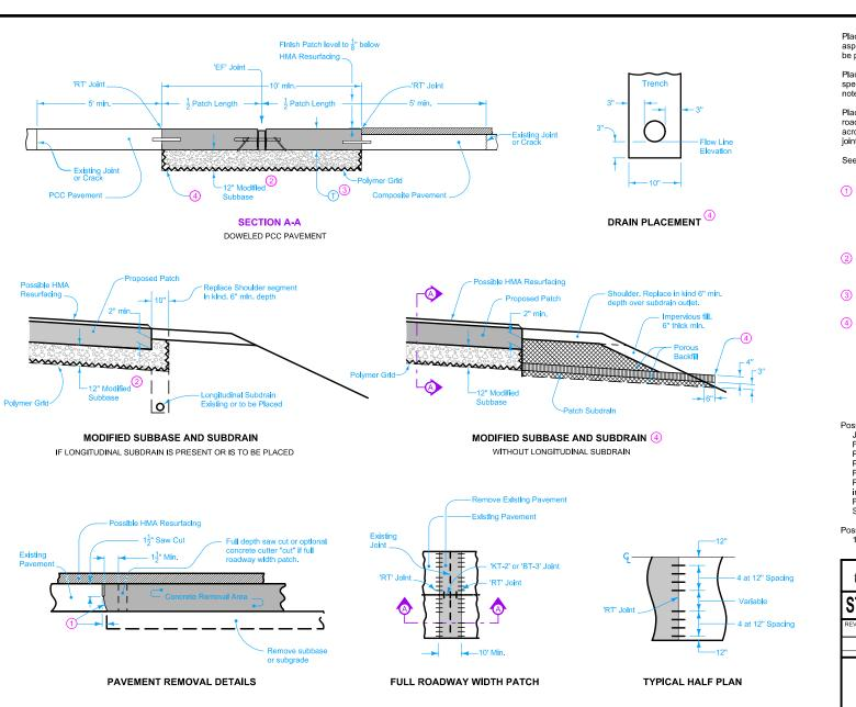
Place Full Depth Patch with 'EF' Joint after the final lift of asphalt has been placed. Porous Backfill and Subdrain may be placed prior to construction of resurfacing of shoulders.
