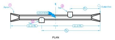
REINFORCED CONCRETE PIPE CULVERT
