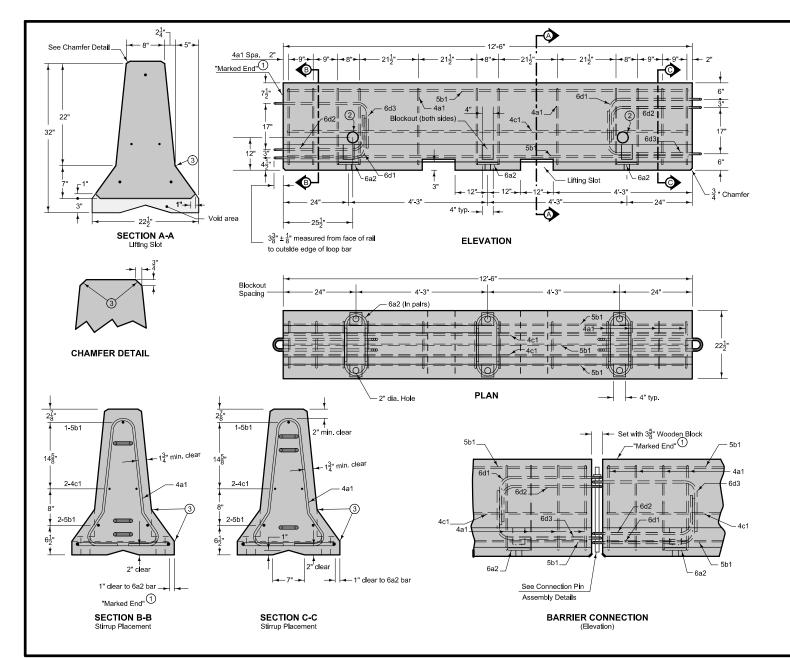
For loop bars 6d1, 6d2, and 6d3, use  $\frac{3}{4}$ " smooth steel bars with a minimum yield strength of 60 ksi, a tensile strength of not less than 1.25 times the yield strength but a minimum of 80 ksi, a minimum 14% elongation in 8 inches, and passing a 180 degree bend test using a  $3\frac{1}{2}$ " pin bend diameter.
