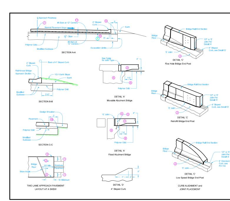
Sections and details apply to Standard Road Plans RK-16 and RK-19B through RK-19J.
