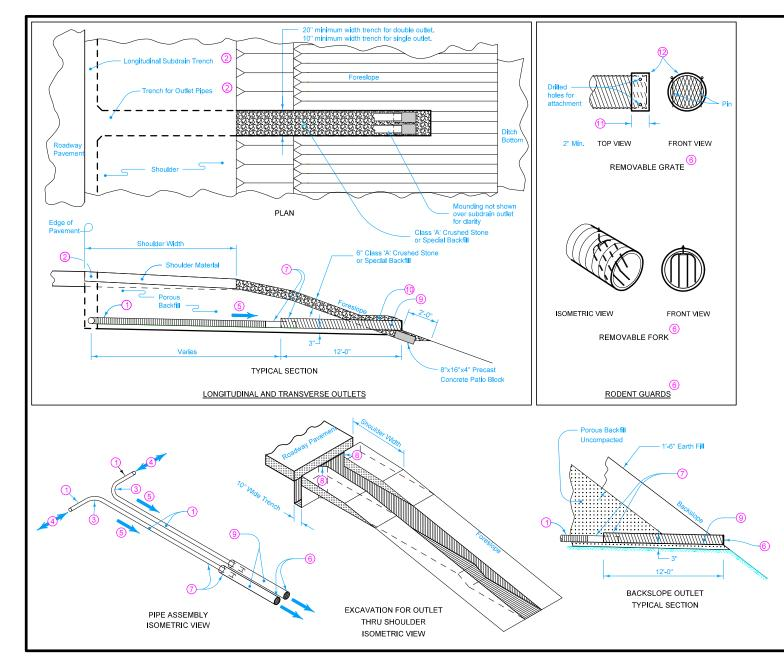
Transverse and backslope subdrains require only single outlets. Install double outlet pipes on all longitudinal subdrain systems, except at the beginning and end of the system. At these locations, install a single outlet pipe.
