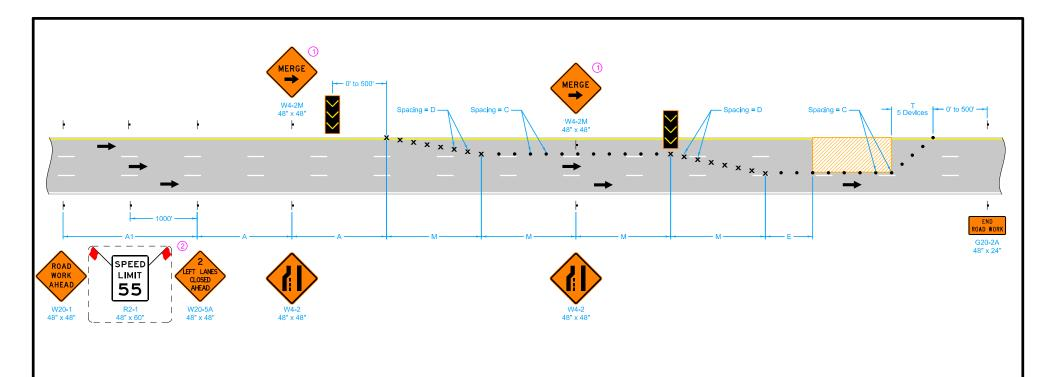
When the Average Daily Traffic (ADT) exceeds 20,000 vehicles per day or when a traffic queue extends beyond the advanced signing, place RIGHT/LEFT LANE CLOSED 4 MILES and RIGHT/LEFT LANE CLOSED 2 MILES signs (W20-5) on both sides of the roadway 4 miles and 2 miles in advance of the lane closure, respectively, as appropriate.
