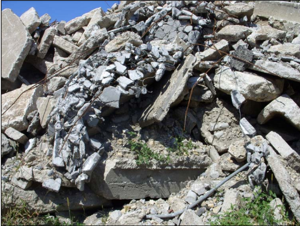
Figure 1. Recycled stockpile contaminated with steel.
