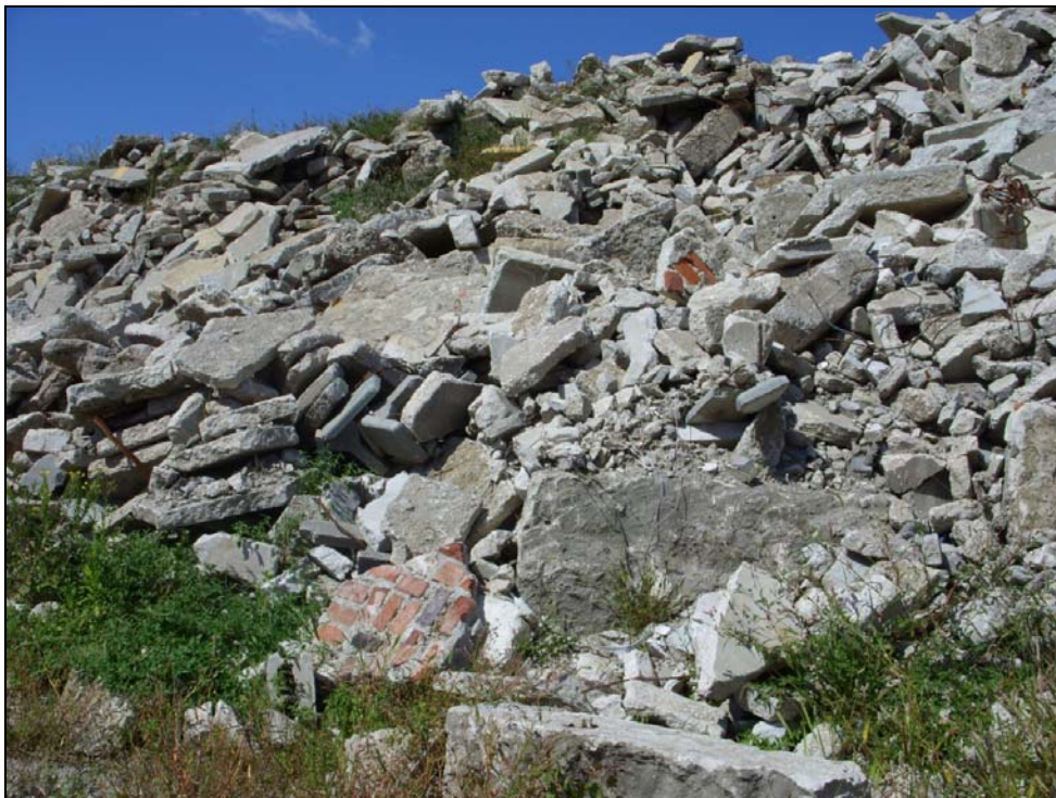
Figure 4. Recycled stockpile contaminated with non-pavement material.
