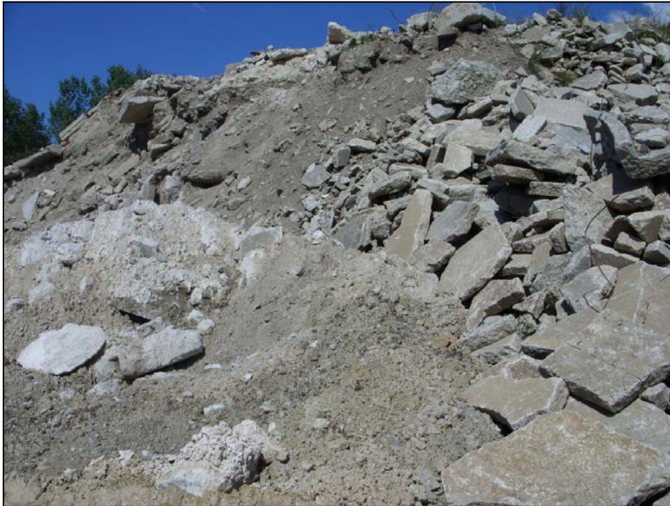
Figure 3. Recycled stockpile with excessive fines.
