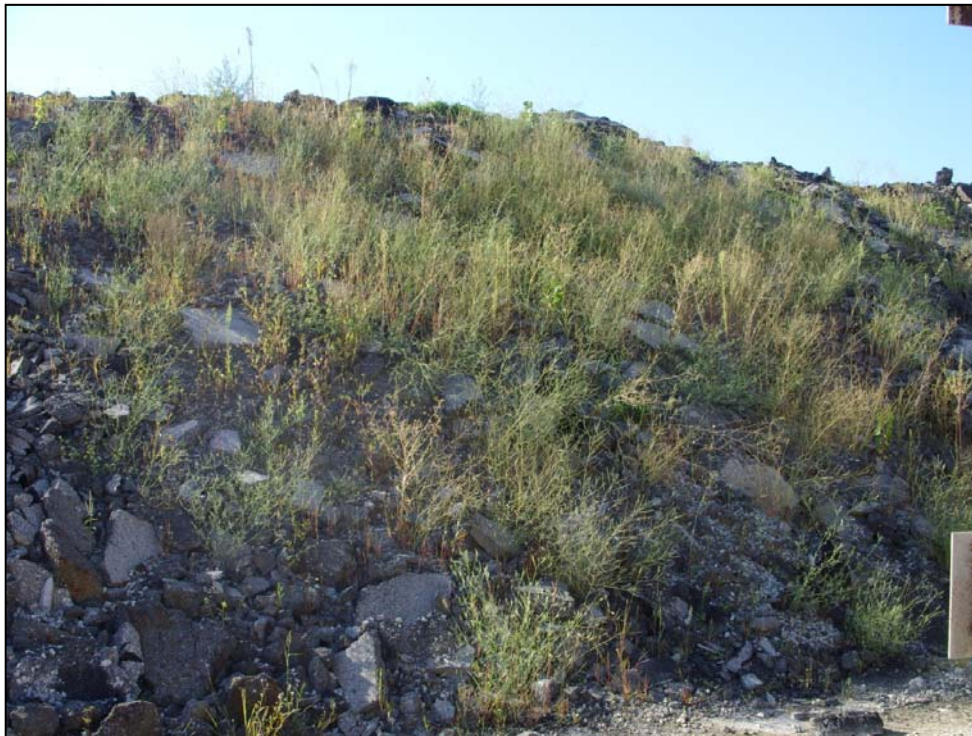
Figure 2. Recycled stockpile contaminated with organic material.
