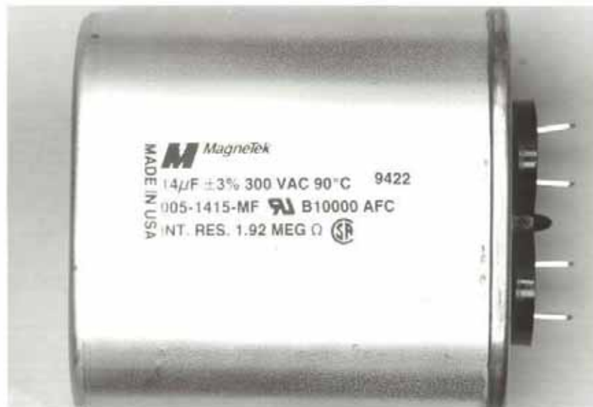
Photograph #8 Capacitor typically found in Mercury Vapor Light ballasts. (PCB statement is found on bottom. Refer to Photograph #9.)
