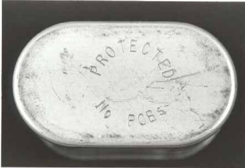
Photograph #9 Capacitor bottom noting the unit is PCB free.
