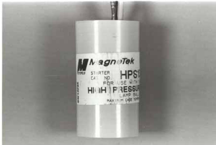
Photograph #10 "Starter" used in Mercury Vapor and Sodium lights. Unit is solid state and contains no PCB's.
