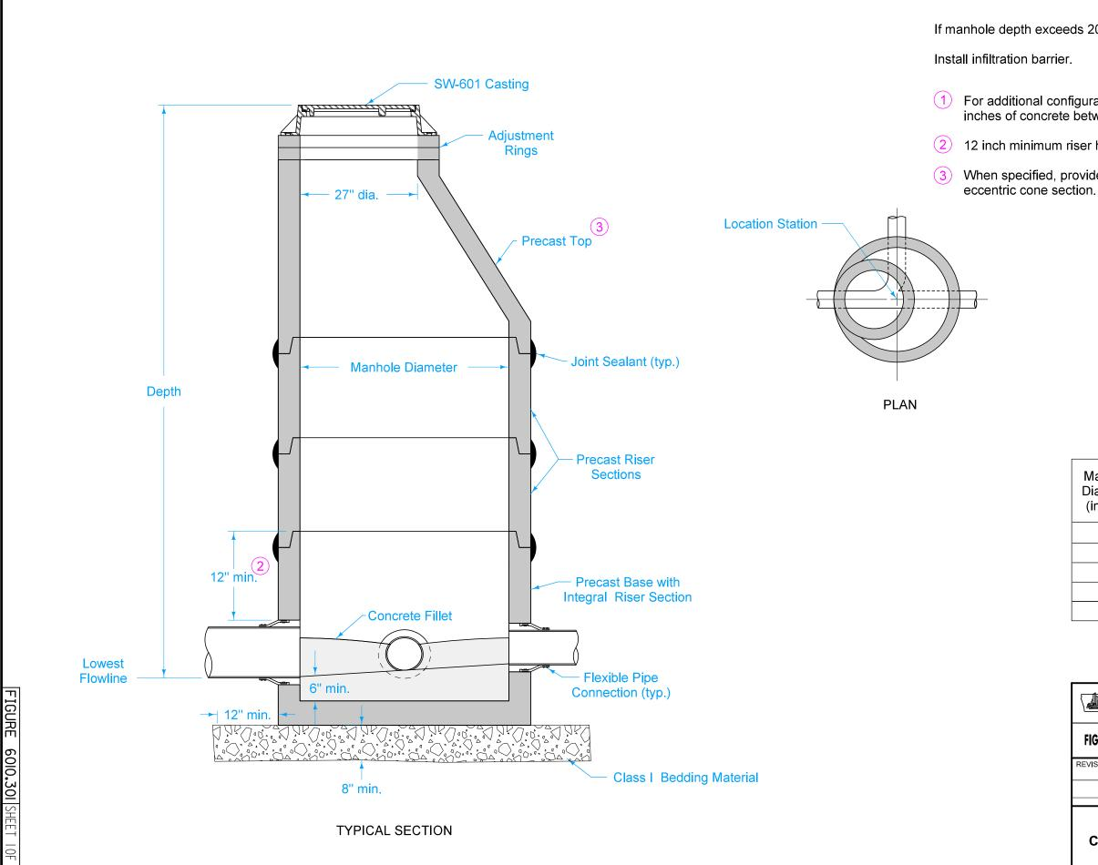
If manhole depth exceeds 20 feet, install steps.
