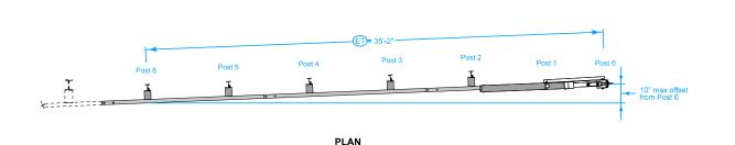
Steel Beam Guardrail Tangent End Terminal 38'-32"
