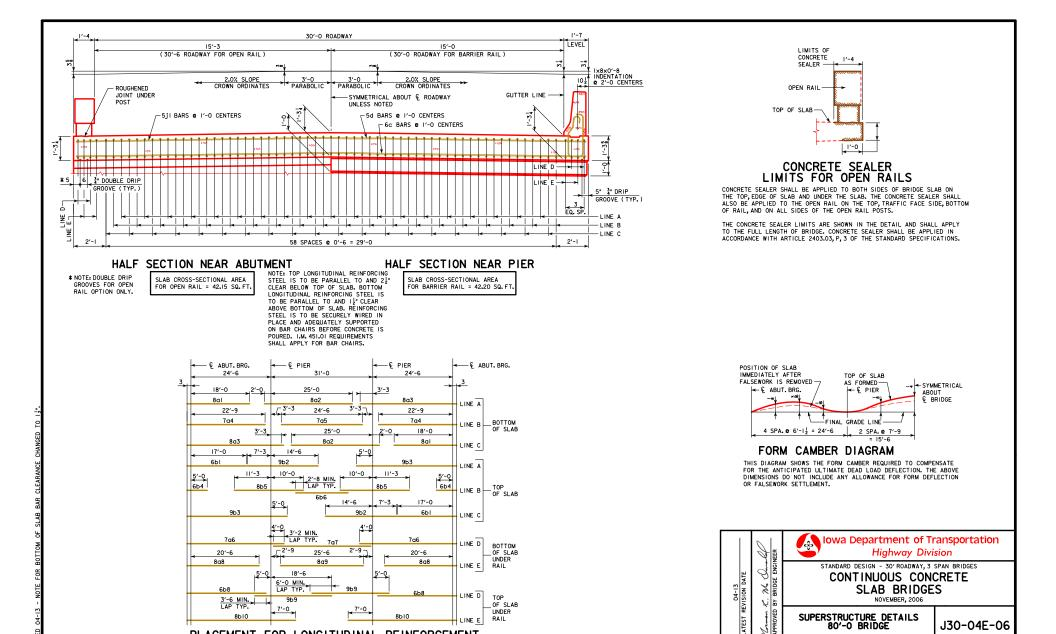
PLACEMENT FOR LONGITUDINAL REINFORCEMENT
