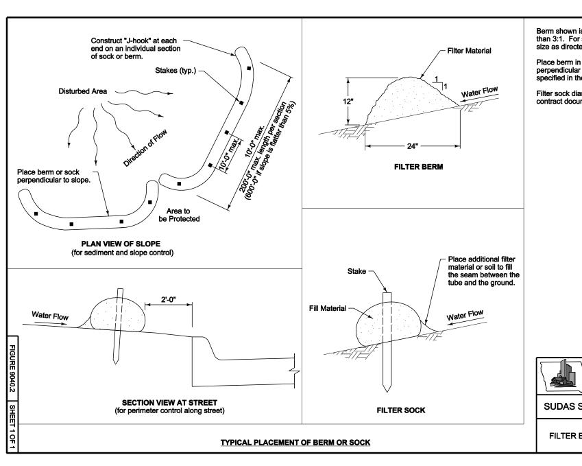
Berm shown is typical for slopes flatter than 3:1. For steeper slopes, increase berm size as directed by the Engineer.
