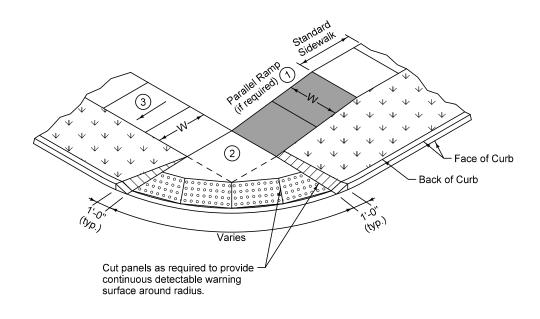
Parallel Curb Ramp: If normal sidewalk elevation cannot be achieved with the perpendicular ramp between the street and landing due to limited ramp length, provide a parallel ramp to make up the elevation difference between the landing and the standard sidewalk.
