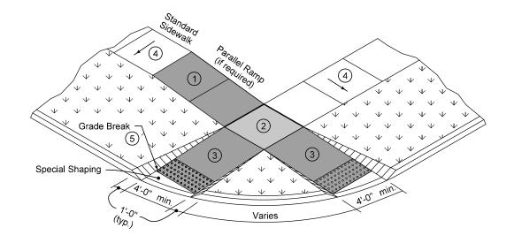
1) Parallel Curb Ramp: If normal sidewalk elevation cannot be achieved with the perpendicular ramp between the street and landing due to limited ramp length, provide a parallel ramp to make up the elevation difference between the landing and the standard sidewalk.
