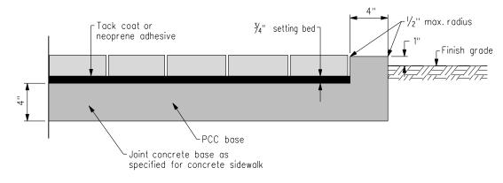
BRICK SIDEWALK WITH CONCRETE BASE
