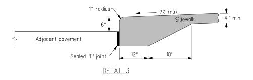
For new sidewalk with new curb and gutter, comply with Detail 1 or Detail 2. Comply with Detail 3 for new sidewalk adjacent to existing povement or when specified in the contract documents.
