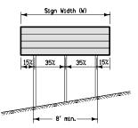
Three Post Erection POST POSITION DETAIL
