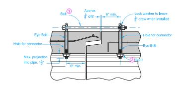
SECTION OF PIPE CONNECTOR (Concrete Pipe to Concrete Pipe)
