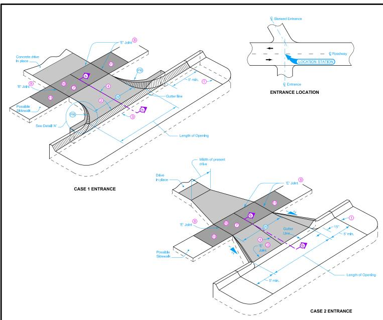
Special details for entrances other than Cases 1 and 2 are included in the detail plans. The shape and surface of driveways and alleys will vary to fit individual conditions.
