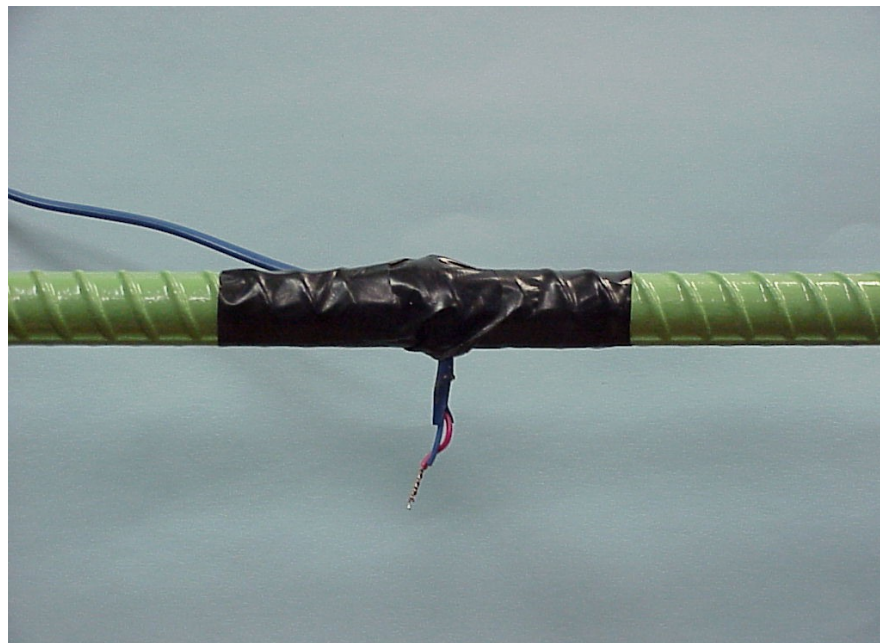
Figure 2. Typical attachment of thermocouple to reinforcing steel
