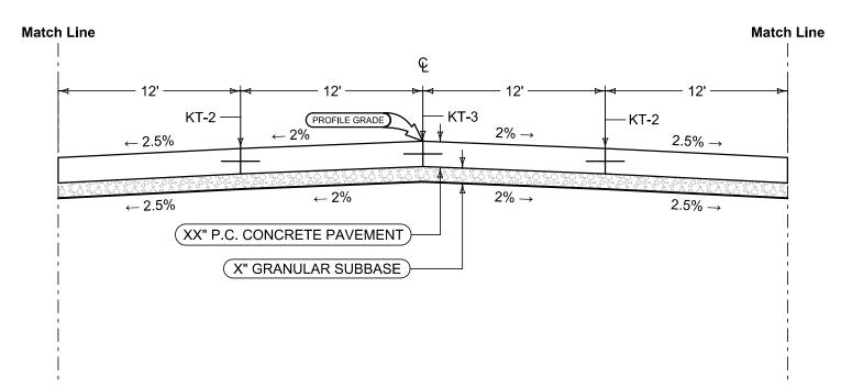
Mainline Jointing: Transverse joints: CD at 17' spacing
