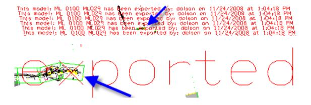
As an additional safeguard, after the **Export** is complete, the program "Locks" the master file model that has been exported, allowing no modifications to the model in the master file while it is exported. After using the **Model\_Export & Import** program to **Import** the model back in to the master file, the program will unlock the model when the import is complete.
