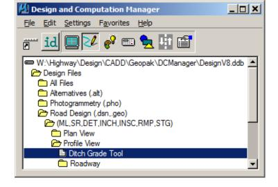
This tool is used to draw correctly formatted ditch grade information into the profile area of a model.
