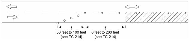
Figure 4: Two-way traffic taper.
