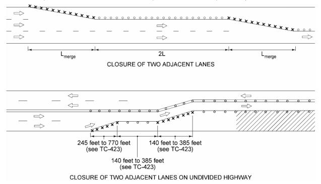
Figure 5: Use of multiple tapers.
