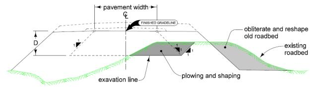
Figure 2: Reshaping roadbed as outlined in Case 2.
