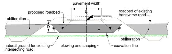
Figure 5: Existing transverse road inside of proposed roadbed.
