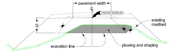
Figure 1: Existing roadbed inside of proposed roadbed as outlined in Case 1.
