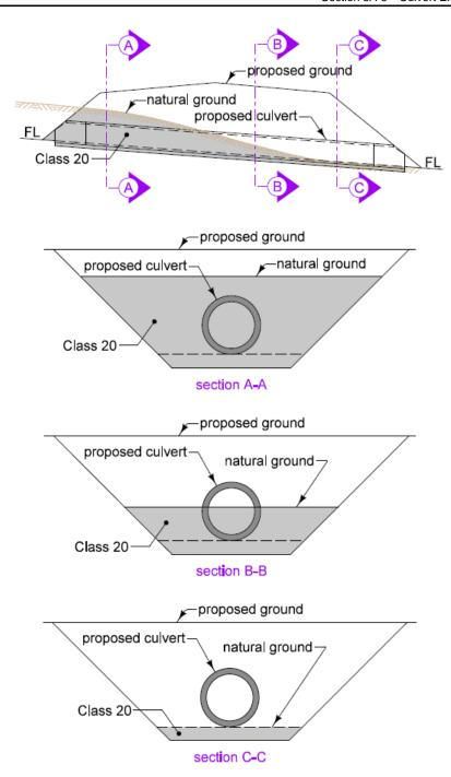
Figure 1: Rigid pipe installation with partial cut.
