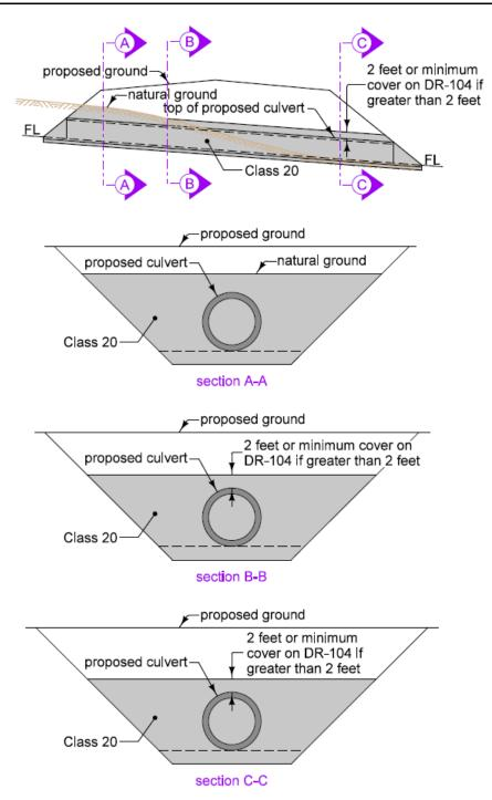
Figure 2: Class 20 for flexible or unclassified pipe installations.
