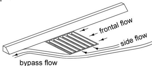
**Figure 3:** Intake bridge end drain flow definitions.
