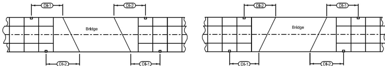
**Figure 1:** DI distances for locating bridge end drains.
