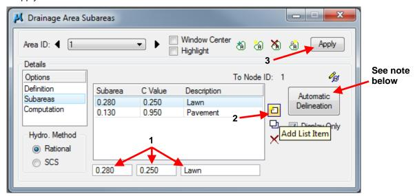
**Note:** To use the *Automatic Delineation* function, line symbology is required to define land use and associated runoff coefficients. The Office of Design has not yet developed this symbology.
