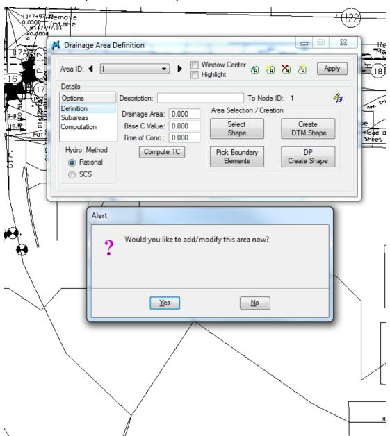
4. Click yes and *Drainage Area* will fill in automatically and the number of the area will appear in the drainage area.
