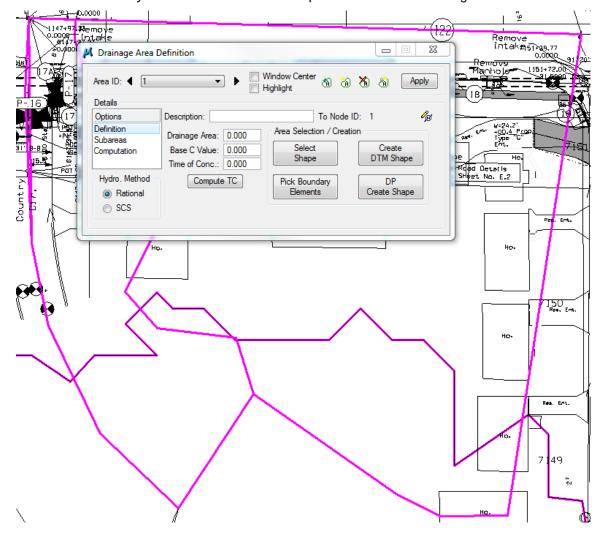
2. Click on *DP Create Shape* (the last element selected will no longer be highlighted) and click inside the drainage area. The area will be highlighted.
