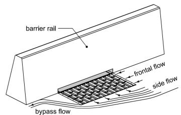
Figure 1: Grate intake flow definitions.
