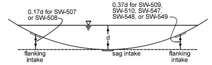
Figure 4: Locating flanking intakes for a sag intake.
