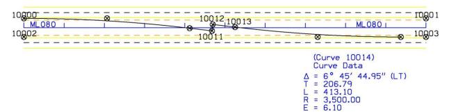
Figure 5: Temporary median crossover geometry for example problem using COGO.
