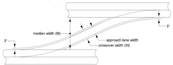
Figure 4: Establishing crossover pavement width.
