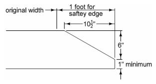
Figure 1: Safety edge dimensions for PCC pavements.
