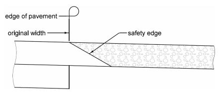
Figure 5: Resurfacing Project without base widening.
