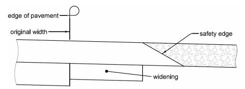
Figure 6: Resurfacing Project with base widening.
