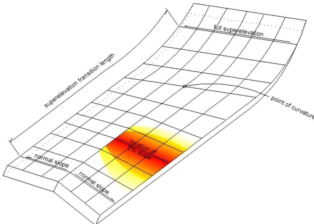
Situations such as this should be avoided if possible. Designers should seek to provide adequate running slope and/or avoid placing the flat location of a vertical curve coincident with the area of no cross slope. However, project constraints occasionally necessitate this occurrence. In these locations, designers should be aware of the implications this holds.
