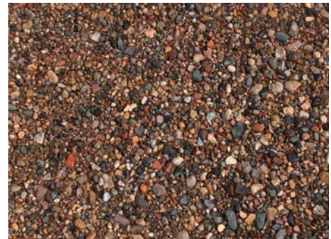
Gravel & crushed gravel as granular subbase
