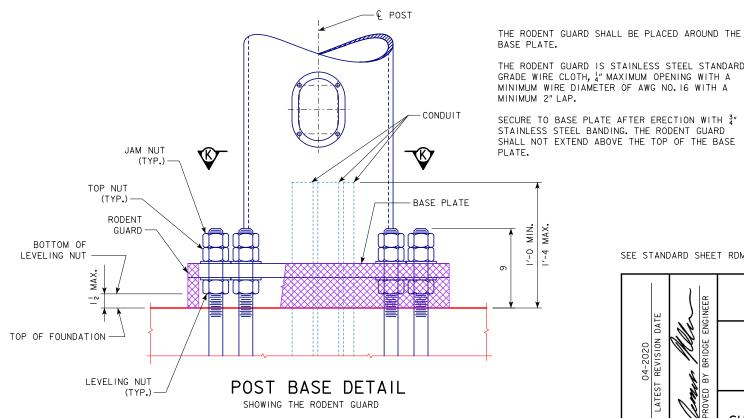
THE RODENT GUARD IS STAINLESS STEEL STANDARD GRADE WIRE CLOTH, 4" MAXIMUM OPENING WITH A MINIMUM WIRE DIAMETER OF AWG NO. 16 WITH A MINIMUM 2" LAP.
