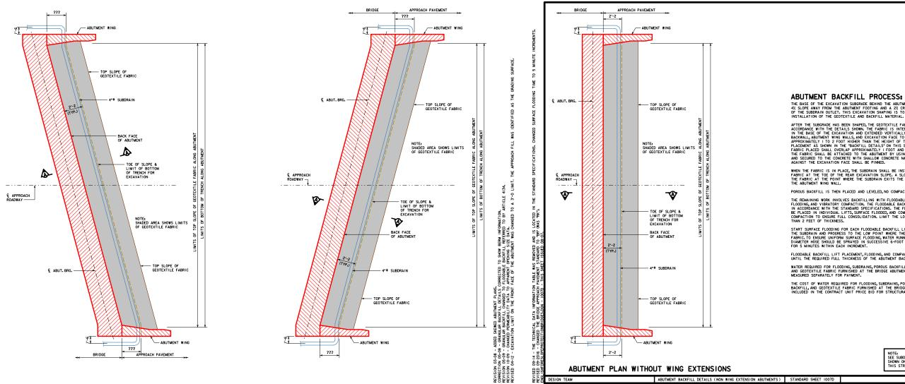
THE BASE OF THE EXCAVATION SUBGRADE BEHIND THE ABUTMENT IS TO BE GRADED WITH A 4% SLOPE AWAY FROM THE ABUTMENT FOOTING AND A 2% CROSS SLOPE IN THE DIRECTION OF THE SUBGRAIN OUTLET. THIS EXCAVATION SMAPHING IS TO BE DONE PRIOR TO BEGINNING INSTALLATION OF THE GEOTEXTILE AND BACKFILL MATERIAL.
