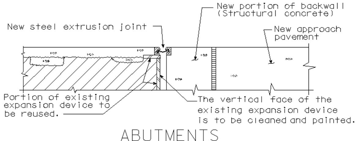
**Figure 12.1.9.1.7. Backwall replacement with remodeled expansion joint**
