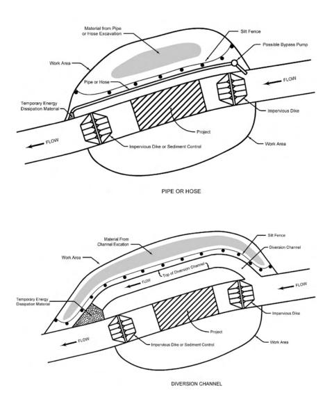
EW-402 provides for different methods the contractor may use to divert flow of a stream. As shown above, a diversion channel is one of the methods. Using a pipe or hose is another method to divert the flow.
