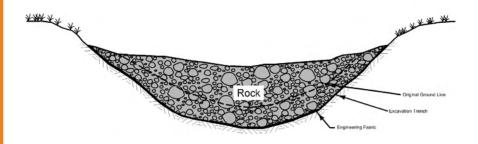
Rock Check Dam detail for temporary applications.
