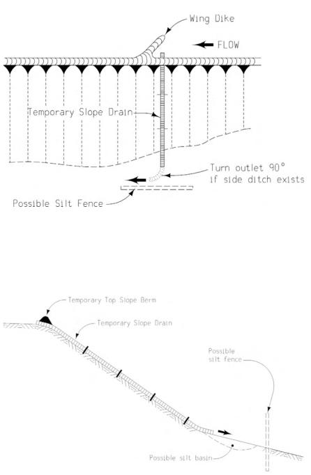
Plan and profile of a temporary slope drain.
