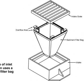
This type of inlet protection uses a sediment filter bag Inlet protection will serve to slow the water down and may result in creating some ponding upstream of the inlet. Because of this, there is potential for inlet protection to create flooding hazards, and these areas should be monitored closely during rain events.
