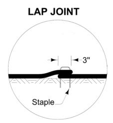
When a new section is added, it should be placed 3 inches over the previous section of fabric and stapled in place.
