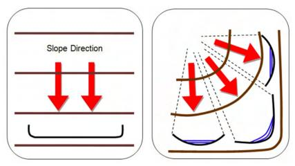
Above illustrations show placement of silt fence along contours of a slope. (The brown lines represent contour lines.)
