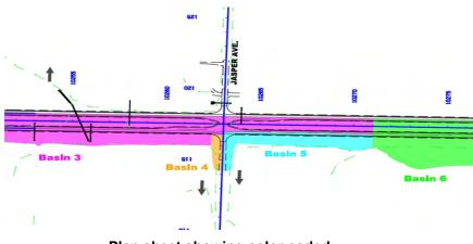
Plan sheet showing color coded drainage basins and discharge points
