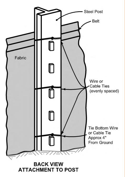
Silt fence fabric is to be attached to the post with three ties.
