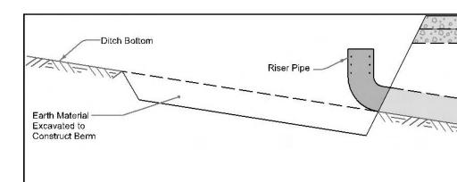
Profile of a temporary sediment control basin.
