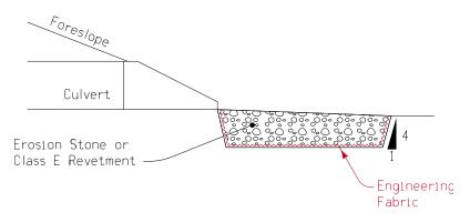
Detail of splash basin at a culvert.
