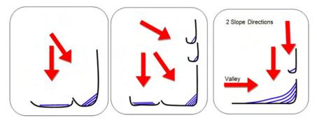
These are examples of correct silt fence placement where a single section of silt fence is broken up into multiple sections with J-hooks. Multiple sections provide multiple storage areas for water to accumulate, thus reducing the chance of a blow-out.
